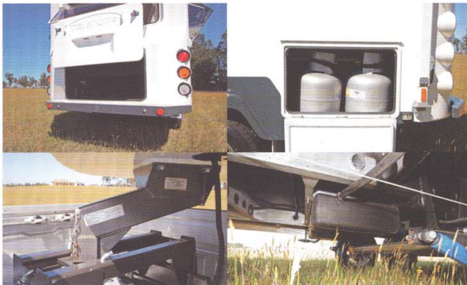
Clockwise from left: Two 9kg gas cylinders; chassis rides on Al-Ko suspension; tow hitch point sits slightly behind axle; rear boot lid lifts up to reveal spacious storage.
