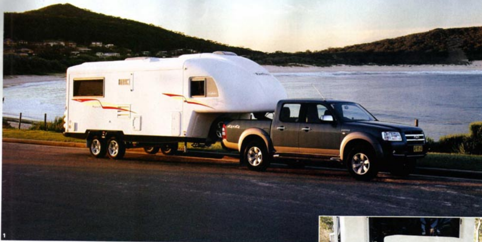
ABOVE 1 Fifth-wheelers, like Travelhome, require a dedicated tow car with tray-mounted hitch installed 2 Rear boot is a useful size and a great addition
