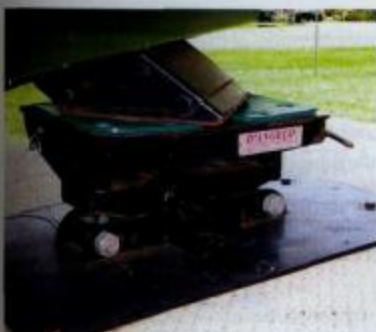
Right top: Single oscillating hitch allows the hitch plate only to revolve (movement not shown) and to rock fore aft.
